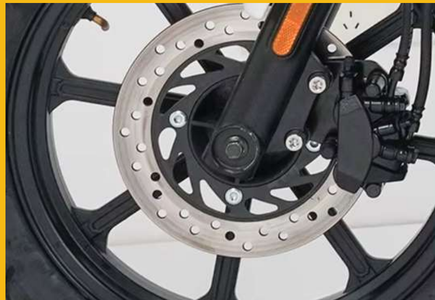
Front disc brake with CBS stability control
