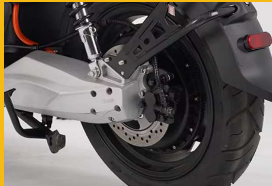
Rear disc brake with CBS stability control
