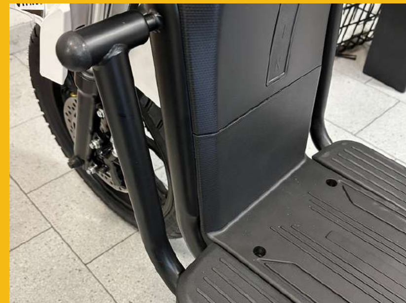
Side protections in case of a fall
